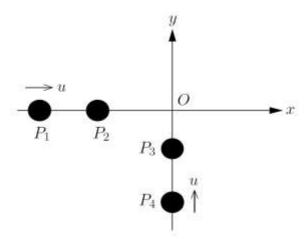
Four particles  $P_1$ ,  $P_2$ ,  $P_3$  and  $P_4$ , of masses  $m_1$ ,  $m_2$ ,  $m_3$  and  $m_4$ , respectively, are arranged on smooth horizontal axes as shown in the diagram.
